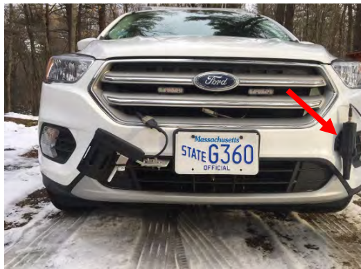
Note: Vaisala MD30 Mobile, Vehicle Mounted RWIS Detectors
