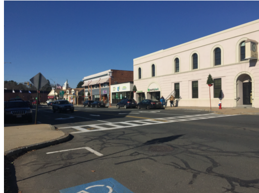
Bumpouts at the Bank Street midblock crossing enhance the visibility of pedestrians and shorten the crossing distance. Adding this feature to other crosswalks on Main Street could further enhance pedestrian safety.
