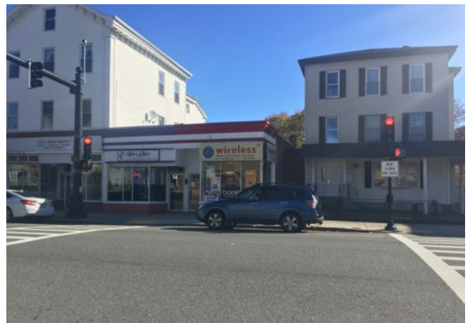
On-street parking within the Harlow Street intersection blocks visibility of pedestrians
