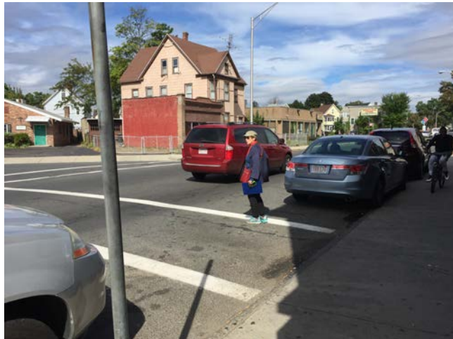
Pedestrians can't see oncoming traffic and drivers can't see pedestrians waiting to cross at the Cleveland Street intersection
