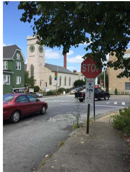
Stop sign is blocked by tree branches and located over 10 feet behind the painted stop line on High Street
