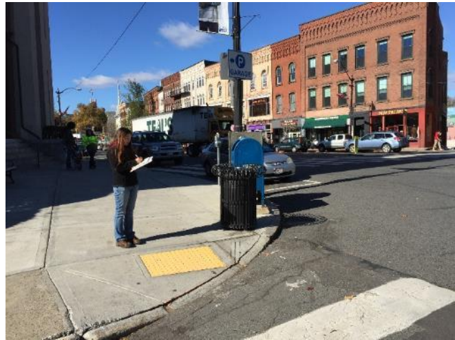
Figure 7 - Parked cars block sight distance for pedestrians at Crafts Avenue.
