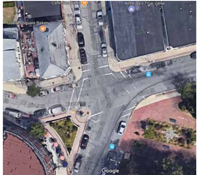
Bolton Street/Rivet Street intersection has long crossing distances and minimal pavement markings.
