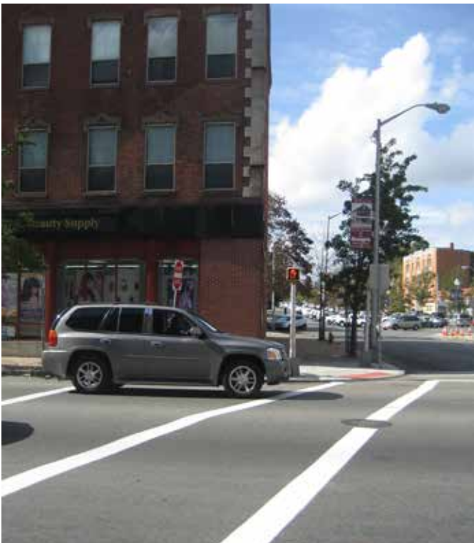
There are two pedestrian push buttons at this location; only one of which controls the signal
